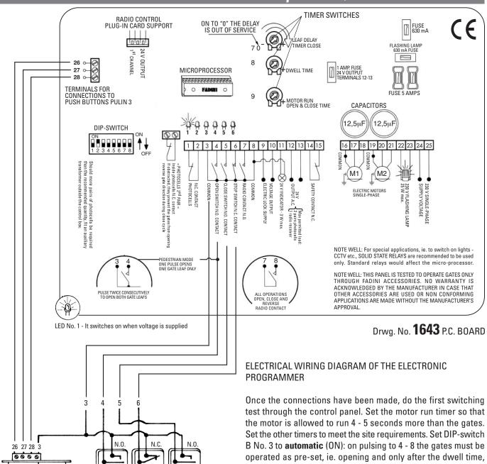
closing. Adjust the times through the respective timers. (See No. 07, 08 and 09 drwg. No. 1643).
