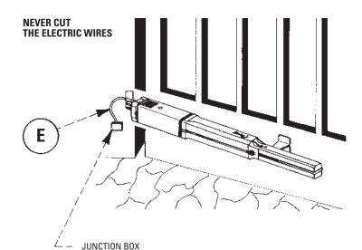
It is essential and most important that the cables "E" are properly removed from their terminal block inside the junction box (Pic.21). Never cut or pull the operator cable away. Also, make sure that the 230 Volt mains switch No. 2 is off. (See page 8, picture 14).
