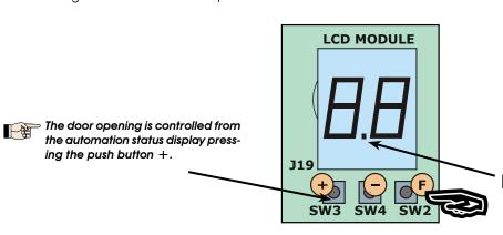
The decimal point indicates that P & H one of the pairs of photocells button is engaged (if enabled on DS1).
