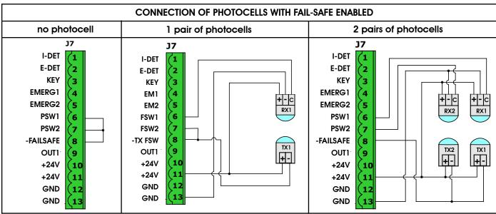
The inputs of the photocells on the connection lay-outs are considered NC contacts (default configuration).
