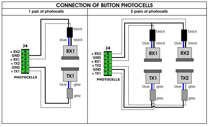
If you are not using any pair of photocells, leave the inputs of connector J4 free.
