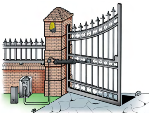
Single mount where 1 ram is required to open/close one gate only
