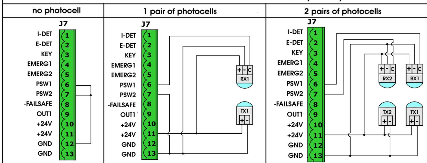
CONNECTION OF PHOTOCELLS WITH FAIL-SAFE ENABLED
