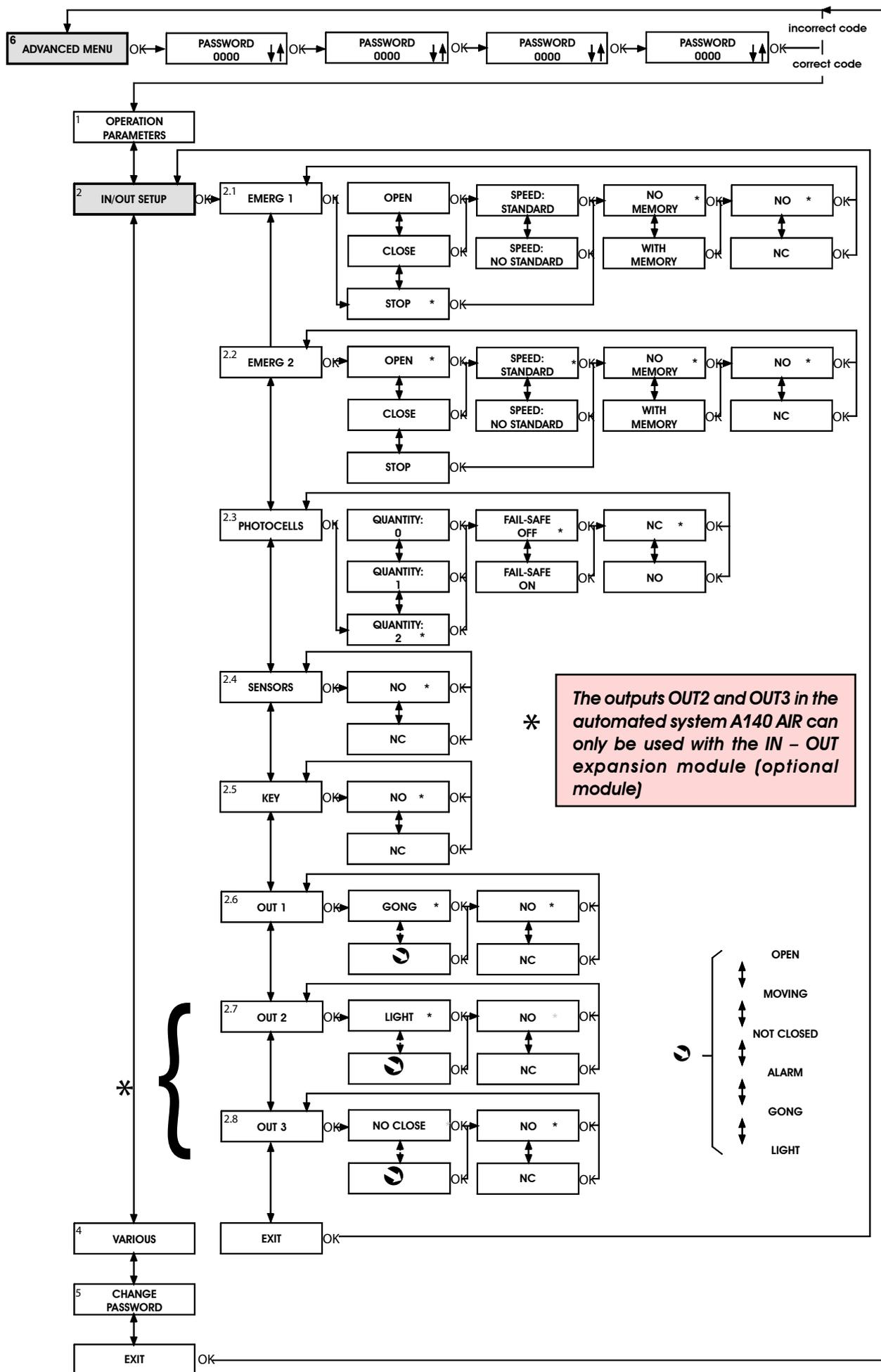
\* The outputs OUT2 and OUT3 in the automated system A140 AIR can only be used with the IN - OUT expansion module (optional module)
