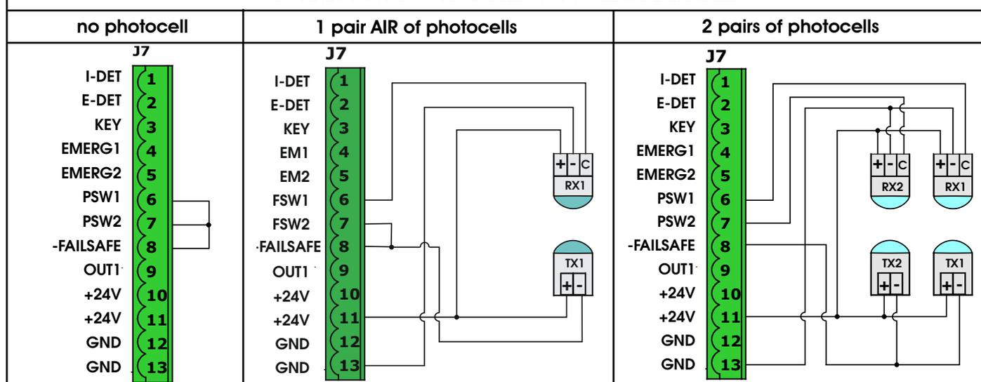
The inputs of the photocells on the connection lay-outs are considered NC contacts (default configuration).
