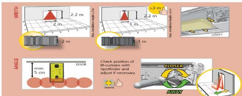
TIP: Launch an ASSISTED SETUP to verify wiring, position of the curtains and correct functioning of the sensor.
