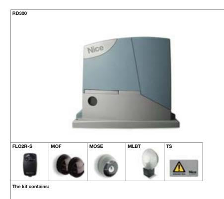
**RD300** 1 irreversible electromechanical gear motor, 24 Vdc, with incorporated control unit and receiver. **FLO2R-S** 1 transmitter 433.92 MHz, 2 channels. **MOF** 1 pair of photocells for outdoor installation. **MOSE** 1 key selector switch for outdoor installation. **MLBT** 1 flashing light with integrated aerial. **TS** 1 signboard.
