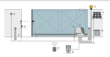
Run 2. Transmitter 3. Photocells mounted on posts 4. Photocells 5. Flashing light
