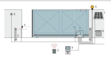
Robus 2. Transmitter 3. Photocells mounted on posts 4. Photocells 5. Flashing light
