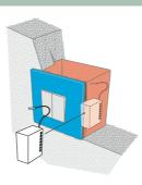
Disappearing inside standard wall mounted plates and suitable to confined spaces, are ideal for restorations and upgrades of existing systems to control home automations, lighting points and all loads up to 500 W not directly accessible from cable controls.
